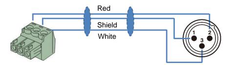
For unbalanced line output connections:
